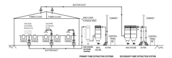
Induction furnace & arc furnaces are offered to control their resulting pollution control by excitraction throl swilling! water cooled hoods or third hole. The extracted hot furnes & gases (often fame loaders) are taken away to TECHFLOW furnace pollution control system consists of Primary air water core! & family throl a pulsajet or reverse air bag house. A powerful ID fan & duct-stack system is provided as ordered.
